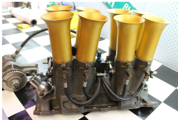
Constant Flow Manifold Injection System
