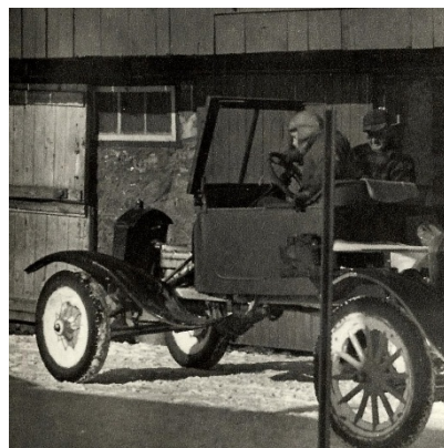
Bill's stripped down Model T with the windshield replaced by a storm window, part of the effort to reduce weight
