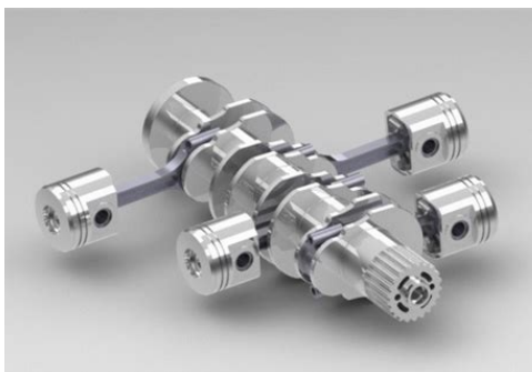
Figure 2: The flat "boxer" 4 cylinder. Click on the photo for an animation
