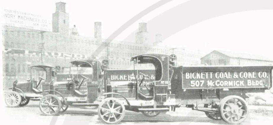
Bickett Coal and Coke Company, Chicago, Ill. The three Pierce-Arrow trucks used by this company are delivering coal direct from standard gondola cars on team tracks. This work is done most economically through the use of a Patented Hopper loading device. One of these trucks recently made a record delivery of 234 tons of coal in one 10-hour day.
