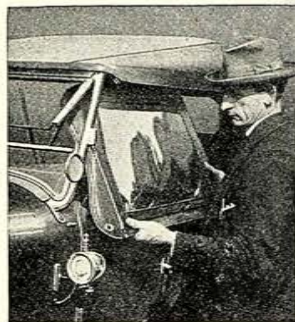
Fig. 38. Fixing front Side Curtain.
