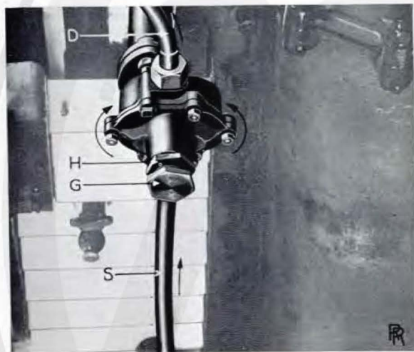
FIG. 5. THE ENGINE OIL PUMP, SHOWING DIRECTION OF OIL CIRCULATION.
