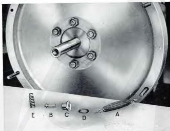
FIG. 10. CLUTCH OIL VALVE DISMANTLED.
