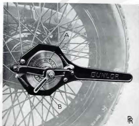
FIG. 24. WHEEL HUB SPANNER IN POSITION.
