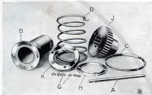
FIG. 28. DETAILS OF REAR HUB.
