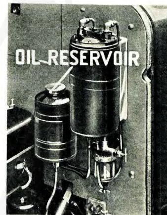
Fig. 31. Showing Oil Reservoir.
