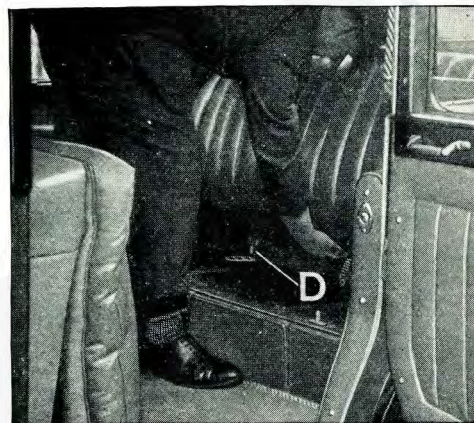
Fig. 33. Showing Adjustment for Rear Squab.
