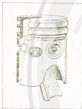
Piston shown in part section.
