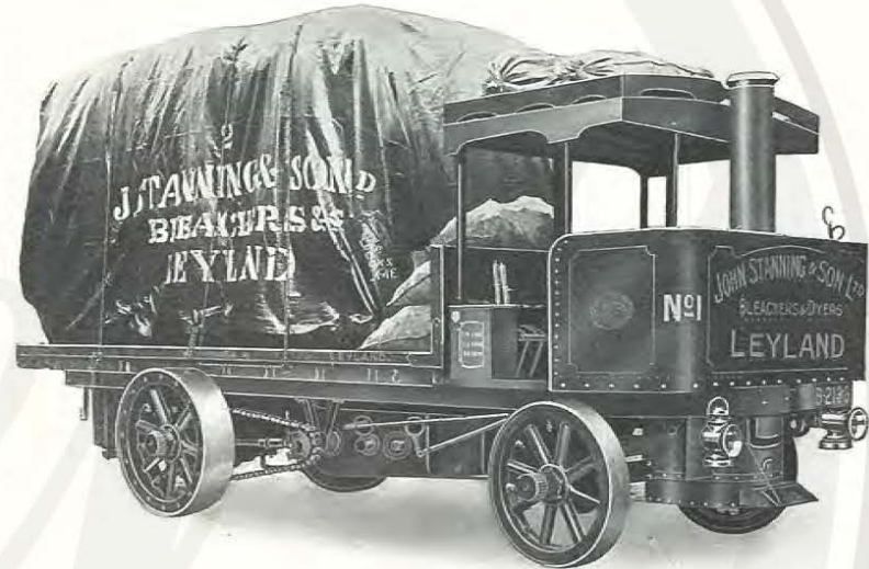
No. 1 Leyland Steam Wagon belonging to Messrs. John Stanning & Son, Ltd. One of the two steamers tested under service conditions by our representative on July 21st last.
