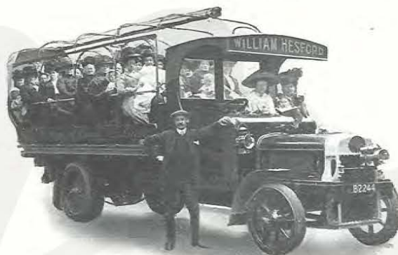
4-Ton Lorry, with Garden Seats and Canopy on Frame, seating 37.
