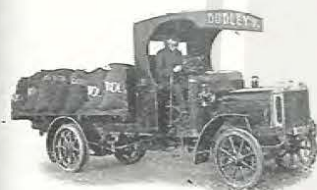
As 30-cwt. Coal Lorry. Body interchangeable with one opposite.
