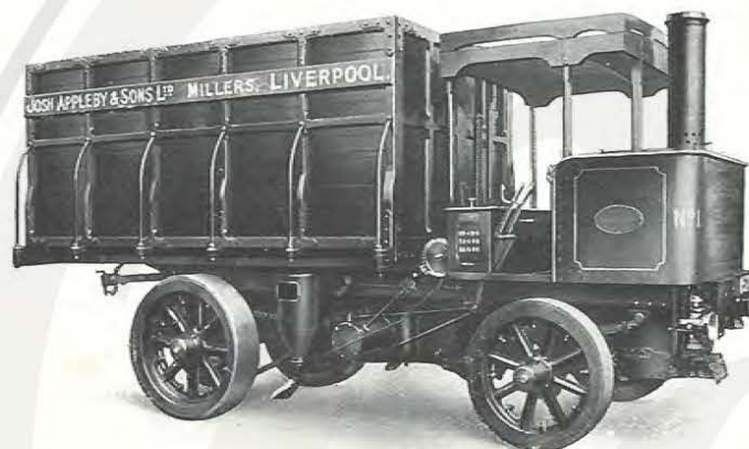
5-Ton Mechanical Tip Wagon, with deep body and sand boxes.
