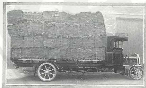
3-Ton Petrol Wagon, with large platform area for hay and straw.
