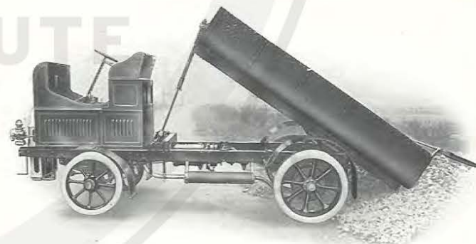
5-Ton Tip Wagon with Steel Body for road material.
