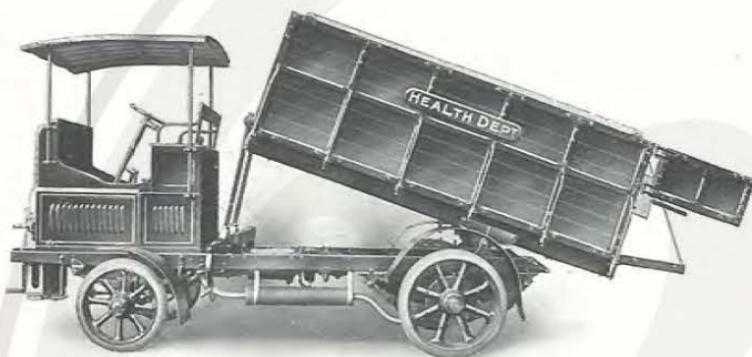
4-Ton Petrol Tip as supplied to Bombay.
