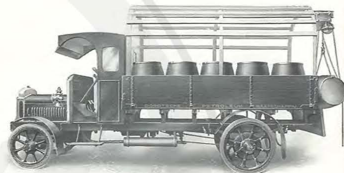
3-Ton Wagon with Self-contained Crane for barrel lifting.
