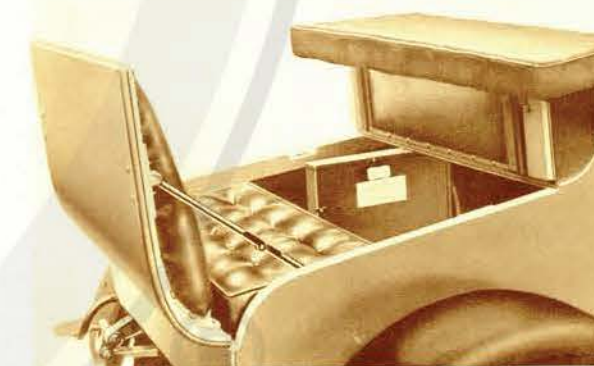
Dickey Seat open, showing location of Battery
