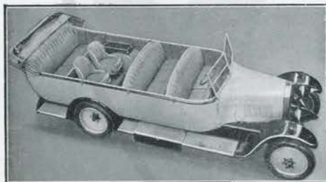
The 14-seater Charabanc on the 30 cwt. low-loading chassis.
