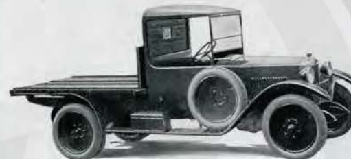
25-CWT. AND 35-CWT. PLATFORM BODIES.
