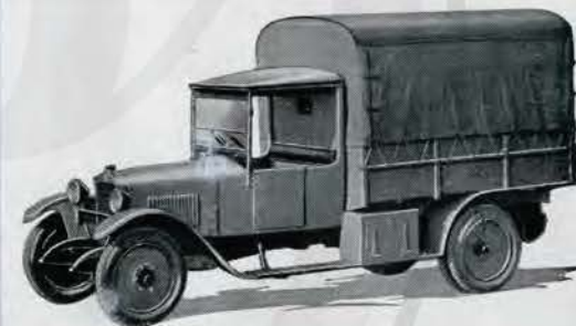
25-CWT. AND 35-CWT. STANDARD BODIES WITH TILT SHEET
