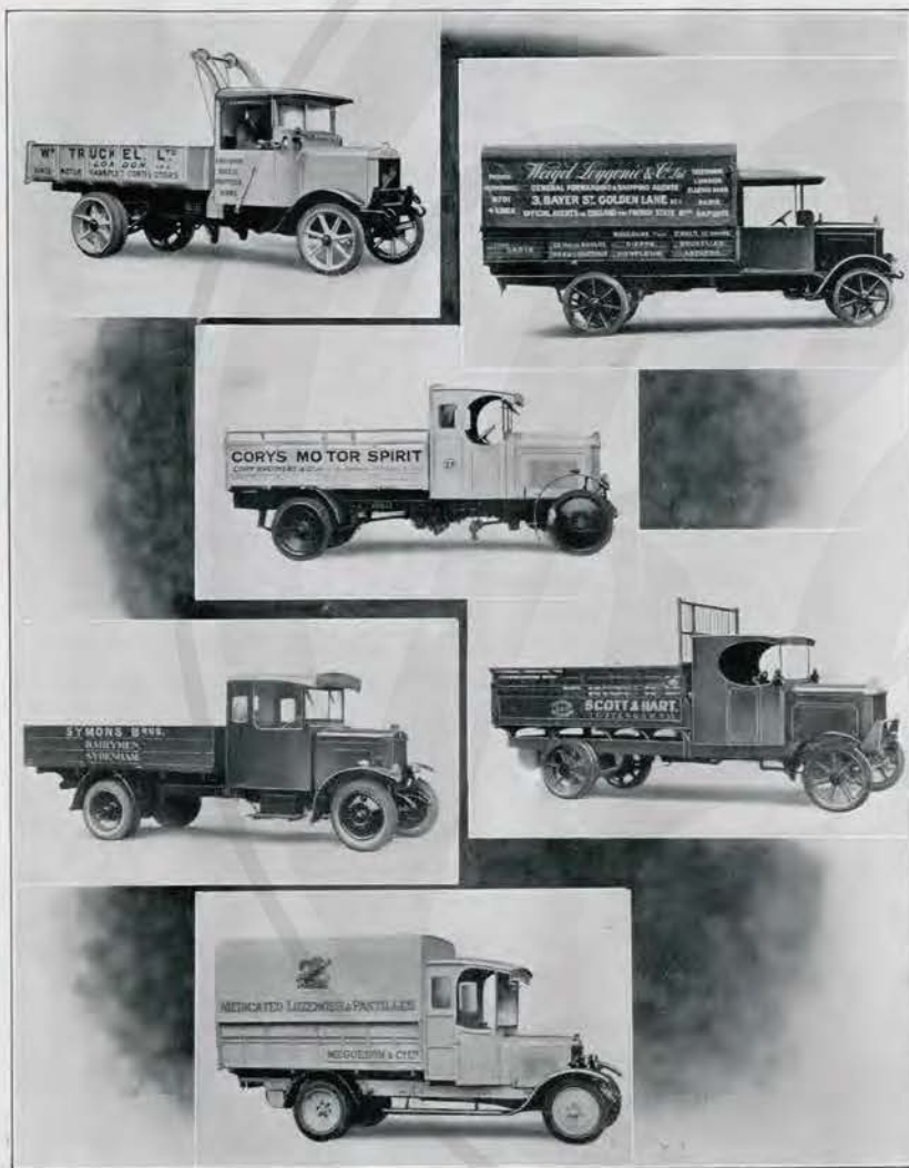
1.—Standard 5-Ton Mechanically-operated Tipper. 2.—Standard 5-Ton Lorry. 3.—Special body on 50-cwt. Chassis. 4.—Drop-sided body on 45-cwt. Chassis. 5.—Special "Covent Garden" body on 3½-Ton Chassis. 6.—Special delivery body on 35-cwt. Chassis.
