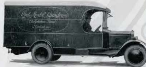
LAUNDRY VAN ON LOW LOADING CHASSIS.
