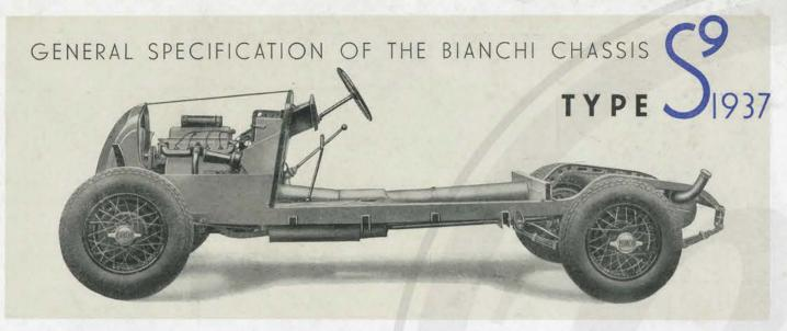
Frame stamped with best quality steel, with cross members of special design making a very rigid chassis
