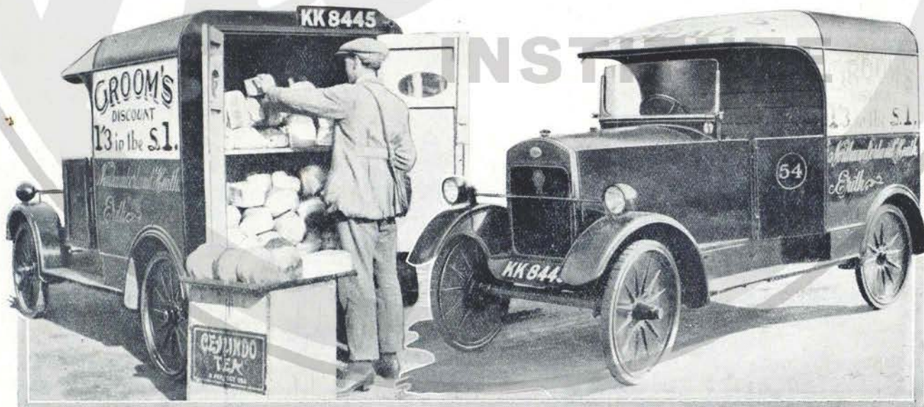
Some idea of the size of the Trojan van may be obtained from the left-hand illustration, and the right shows the partition that has been built in by Grooms to keep the load separated from road dust.
