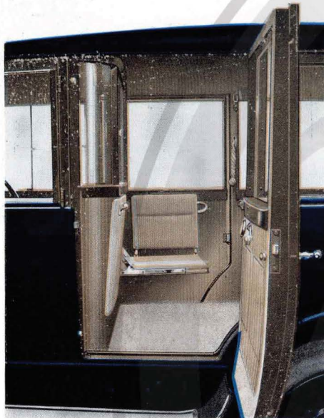
A glimpse through the rear door of an 18 h.p. closed body showing one of the folding seats.
