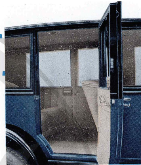
The rear compartment of the Saloon body on the Short 18 showing the wide doors and drop windows.
