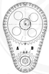
Fig. 26. Crankshaft and Camshaft Sprockets with Chain.
