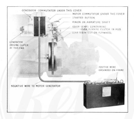
Fig. 32. Motor Generator and Starting Mechanism.
