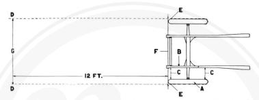
Fig. 53. Diagram Showing Method for Aligning Front Wheels.
