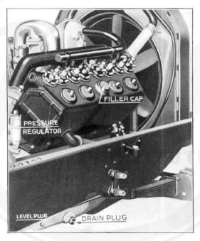
Fig. 18. Oil Filler Cap, Pressure Regulator, Level Plug and Drain Plug.
