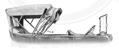
Fig. 10. Top Partially Folded, 2nd Position.
