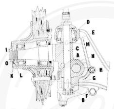
Fig. 51. Front Left Spindle and Hub, Showing Bearings.
