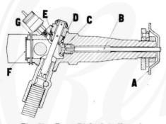
Fig. 52. Front Right Spindle and Speedometer Driving Gears.
