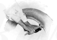
Fig. 62. Placing Tire on Rim, 4th Position.
