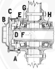
Fig. 47. Sectional View of Rear Hub, Showing Bearings.
