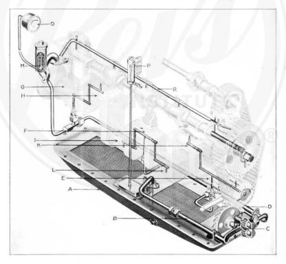
Fig. 17. Engine Lubricating System.
