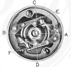
Fig. 34. Timer Contacts, Distributor Cap and Rotor Removed.
