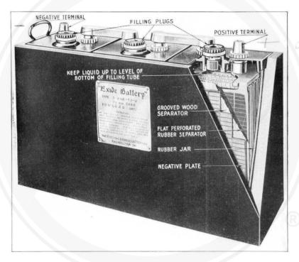
Fig. 36. Storage Battery, Sectional View.
