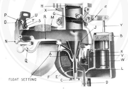
Fig. 22. Carburetor, Sectional View.
