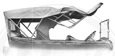
Fig. 13. Top Partially Raised, 2nd Position.
