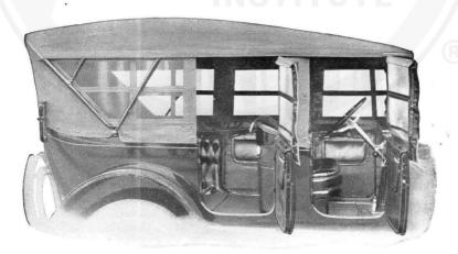
Fig. 14. Side Curtains in Place.
