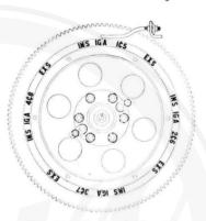
Fig. 35. Flywheel, Showing Timing Marks.
