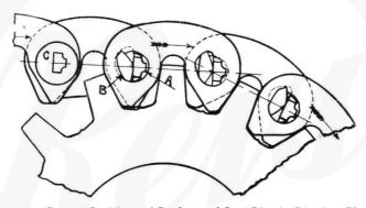
Fig. 27. Correct Positions of Rocker and Seat Pins in Riveting Chains.
