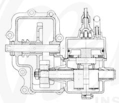
Fig. 45. Tire Air Compressor, Sectional View.
