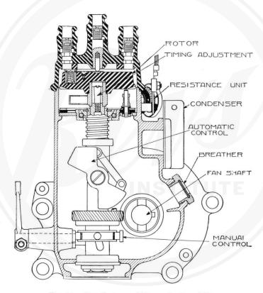
Fig. 33. Distributor and Timer, Sectional View.
