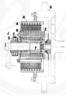
Fig. 41. Main Engine Clutch, Sectional View.
