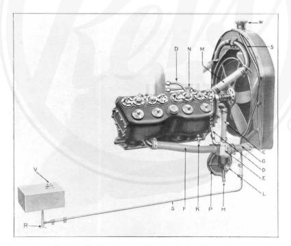
Fig. 24. Cooling System, Showing Path of Circulation.
