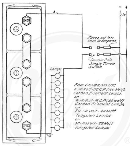
Fig. 38. Diagram of Connections for Charging Battery from 110 Volt D. C. Circuit.
