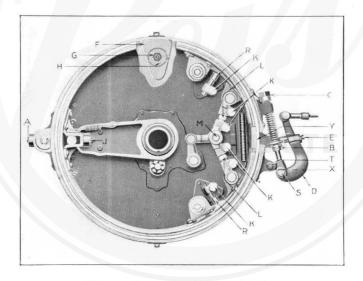
Fig. 48. Internal and External Brakes.
