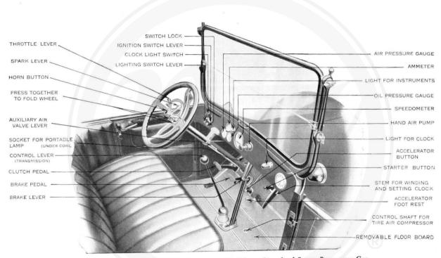
Fig. 1. Instruments, Control Levers and Pedals on Standard Seven Passenger Car.
