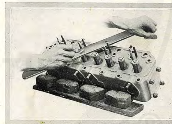
Illustrating a simple method of removing a valve described on the next page. The cylinder head is laid on four specially shaped blocks of wood similar to those shown and thus prevents the valve from sinking when the spring is depressed in the manner shown.
