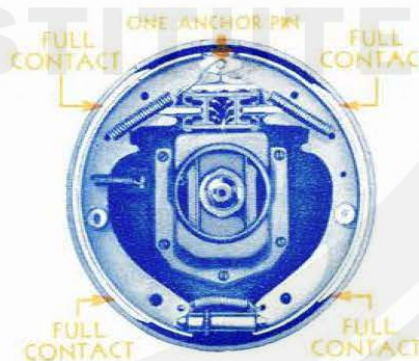
Buick brake with full shoe contact at top and bottom
