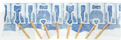
Buick valve seats individually cooled
