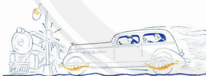
In the conventional car, the burden of all braking loads is placed on the springs
