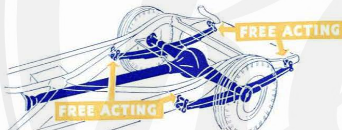
Buick rear springs are "free acting" at front and rear, made possible by torque tube drive, which pushes the car
