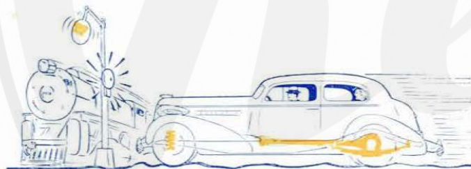
In the New Buick, the Torque Tube and Knee-Action Arms absorb all braking loads
