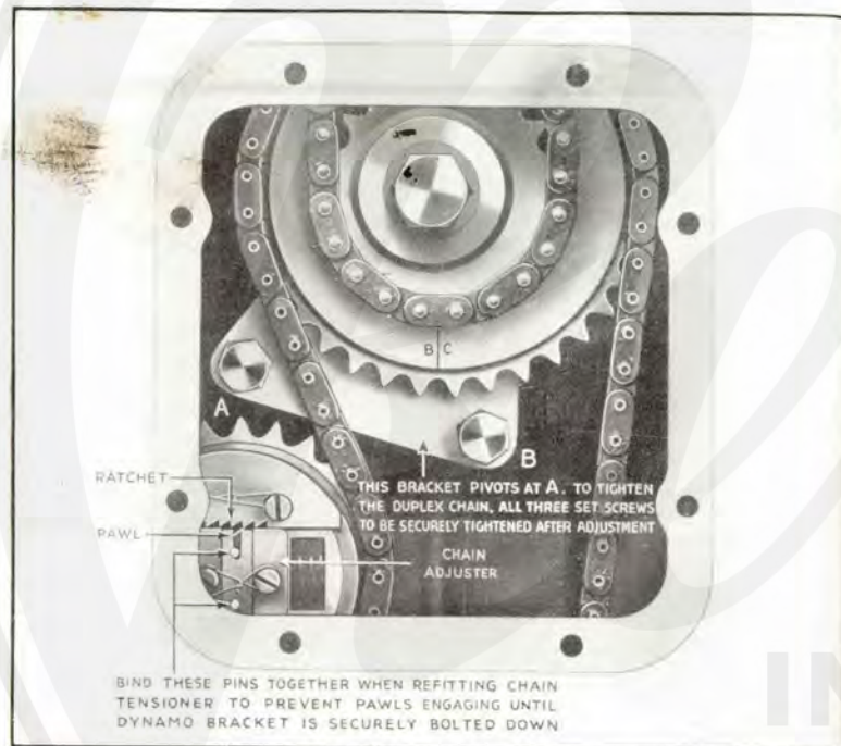
View of Engine Chains, showing Eccentric Bush and Chain Adjuster.
