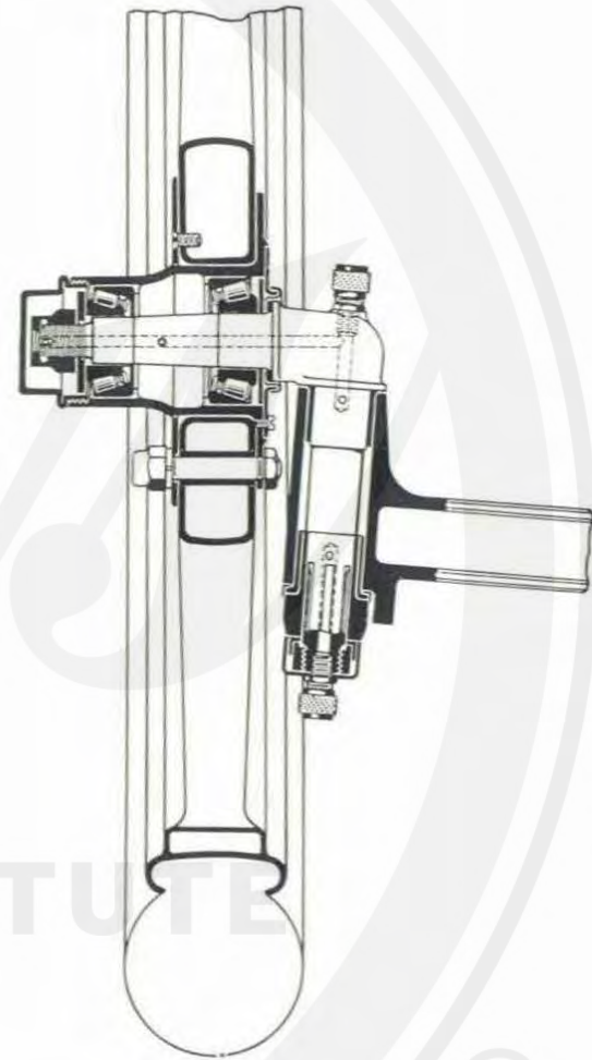
SECTIONAL VIEW OF FRONT HUB AND SWIVEL AXLE.
