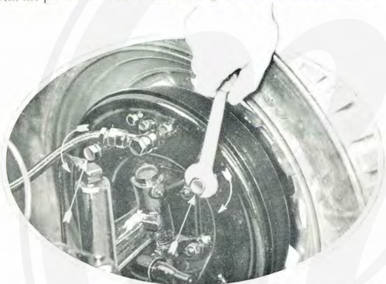
Here are shown the two shoe adjusting nuts to be found on each brake back plate. The small arrows indicate the direction in which they should be turned to bring the shoes closer to the drums.
