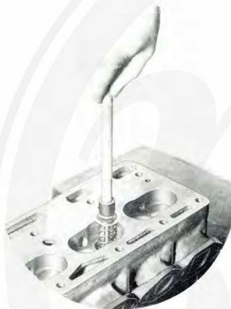
The insertion of a light spring under the valve head greatly facilitates valve grinding.
