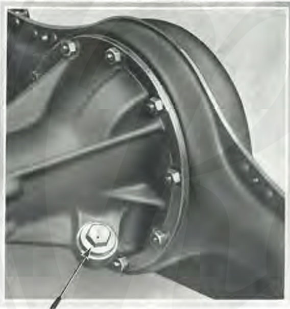
This illustration indicates the combined oil filler and level plug on the rear axle.
