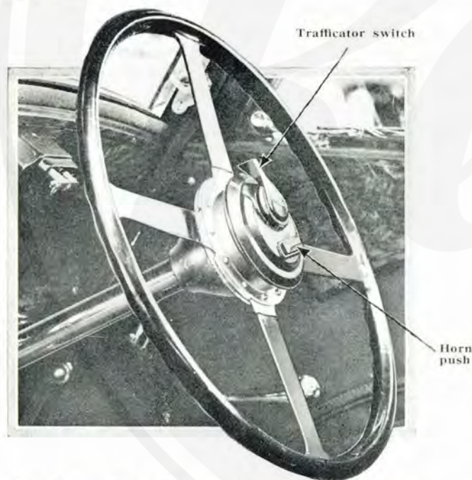
The self-cancelling Trafficator switch and the horn push are mounted in the centre of the steering wheel.
