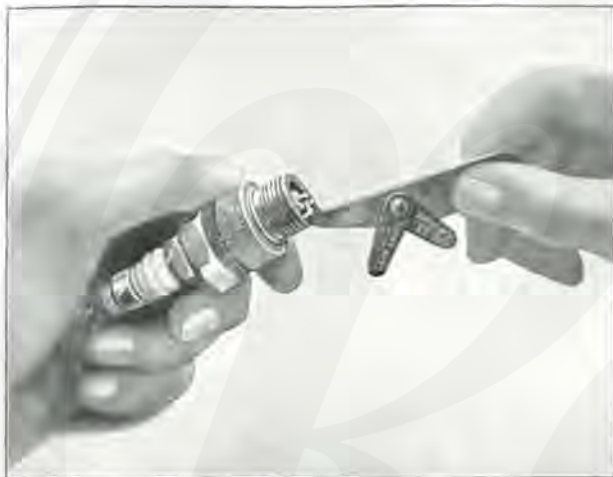
Adjustments should be made only by the side wire, and the combined setting tool and gap gauge illustrated can be obtained from the Champion Sparking Plug Co. or your Wolseley Dealer for 4d.
