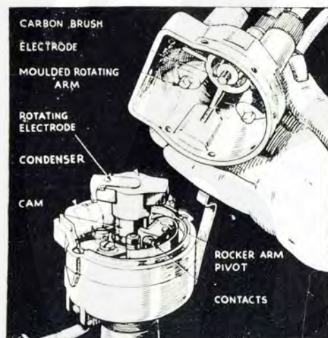
The Lucas distributor with cover removed to show its construction.
