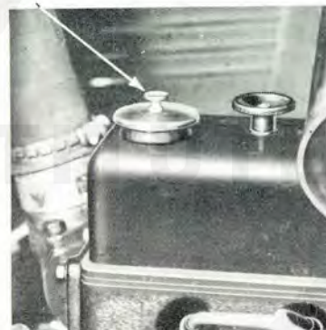
The engine oil filler is accessibly situated in the valve cover of the engine.
