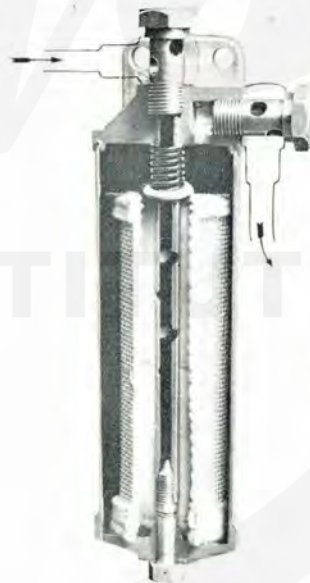
The external oil filter is situated on the left-hand side of the engine, next to the oil pump. In the illustration it is partly cut away to show its internal construction.
