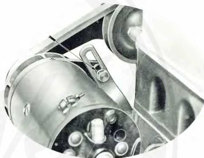
The method of adjusting the dynamo and fan belt.
