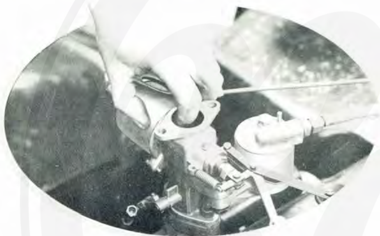
Testing the carburetter piston for freeness.
