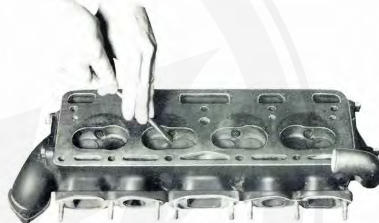
Decarbonising the cylinder head of the Wolseley 12/48.
