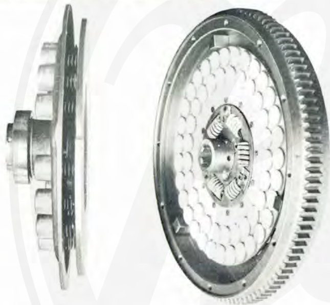
The component parts of the Wolseley 10 40 and 12 48 clutch.
