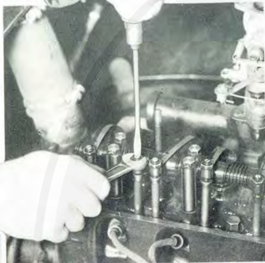
Left :— The tappet adjustment screw is released for adjustment by slackening off the hexagon lock nut with a spanner while holding the tappet screw against rotation with a screw-driver. The tappet screw is relocked in a similar manner after adjustment.
