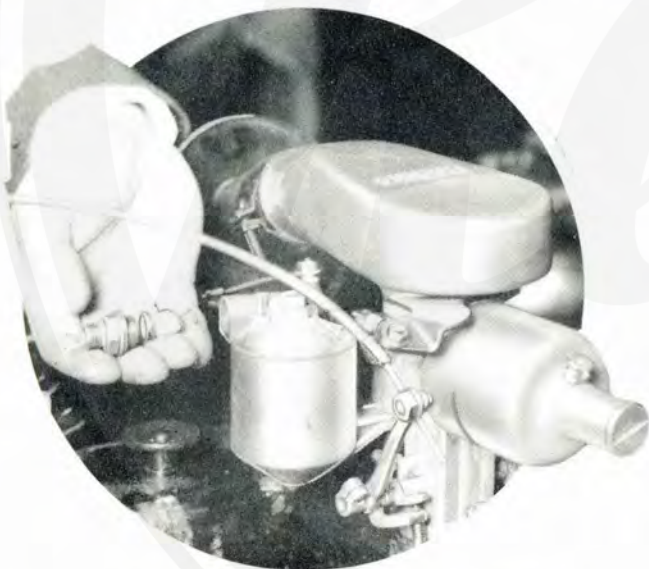
The petrol feed pipe removed to show the filter.
