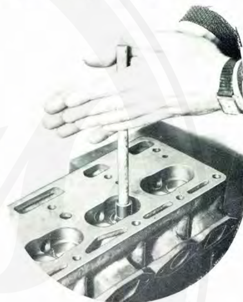
Grinding-in the valves with the help of the special suction tool.
