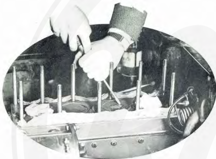
Scraping the carbon from the piston crowns.
