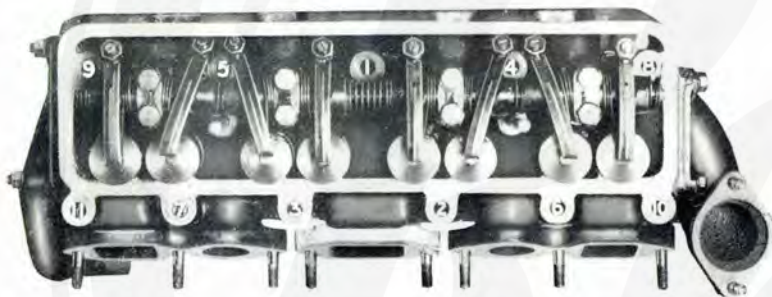
The correct order of tightening the cylinder head stud nuts.
