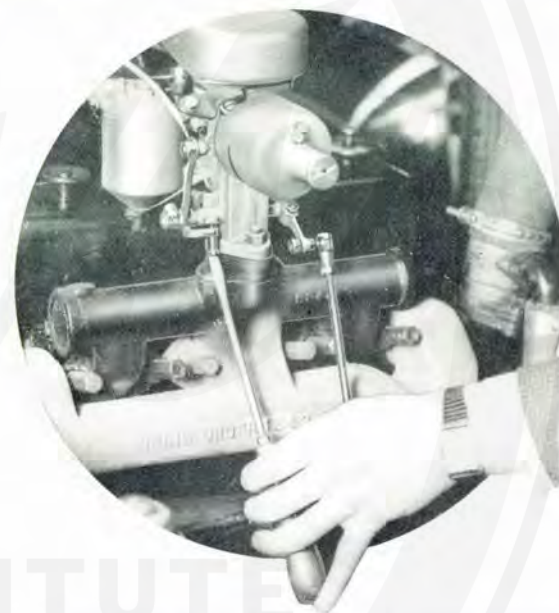
Adjusting the clearance of the dash slow-running control which should be quite clear of the throttle control.
