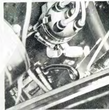
The oil level dip-stick indicator is situated on the near-side of the cylinder block, and is readily accessible.
