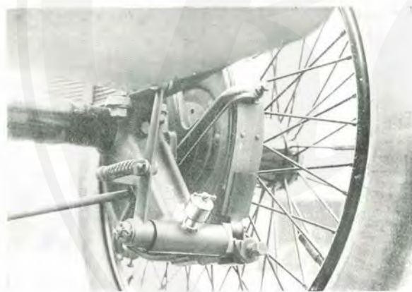
SHOWING ADJUSTMENT AND LUBRICATION OF REAR BRAKES
