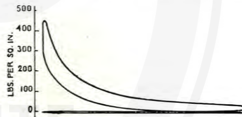
Fig. 29.—Typical Indicator Diagram, "D.H." Type
