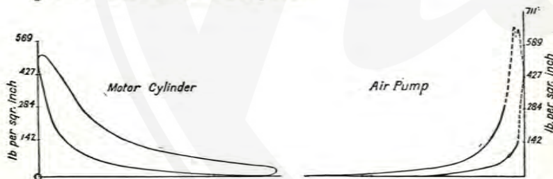
Fig. 34 Indicator Diagrams: Diesel Oil Engine
