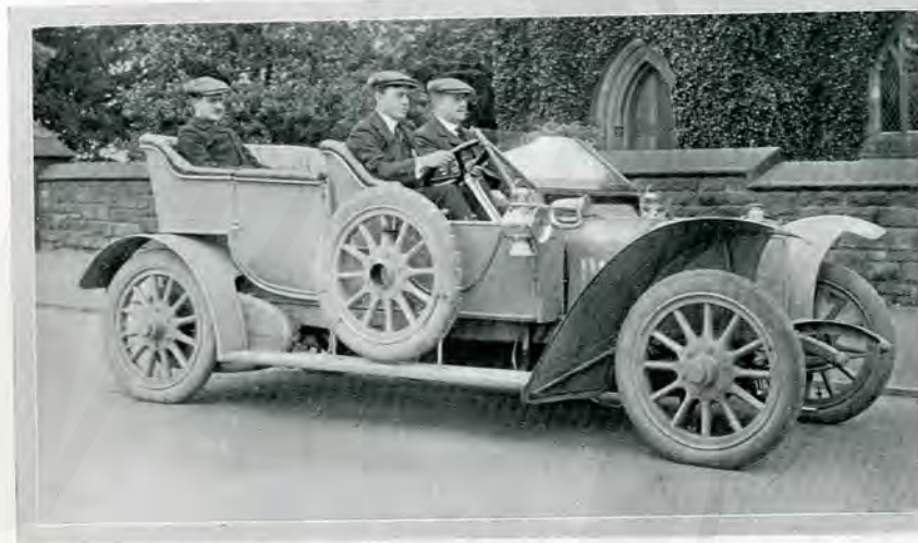
The first Sunbeam car (16-20 h.p.) designed by Mr. L. Coatalen. Only three of this type were built with chain drive, all the remainder being fitted with live axle.
