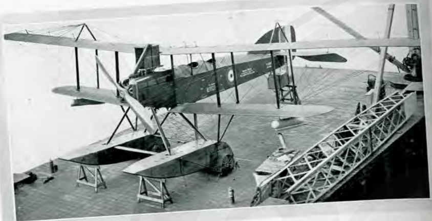
A Short seaplane fitted with Sunbeam-Coatalen aircraft engine. Similar machines carried bags of flour and other supplies to General Townshend's garrison at Kut-el-Amara.
