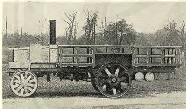
FIG. 23.—THE FIRST THORNYCROFT LORRY WITH INTERNAL COMBUSTION PARAFFIN ENGINE.
