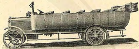
FIG. 62.—X-TYPE 28-SEATED MOTOR COACH.
