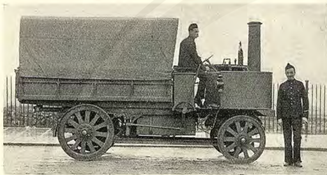
FIG. 22.—THE BRITISH ARMY'S FIRST SELF-PROPELLED VEHICLE, A THORNYCROFT STEAM WAGON OF 1899.
