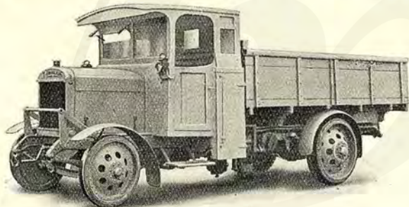
FIG. 55.—J-TYPE LORRY WITH THORNYCROFT SUCTION GAS PRODUCER.
