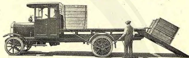
FIG. 65.—HAULING GEAR IN USE ON 4-TON LORRY.
