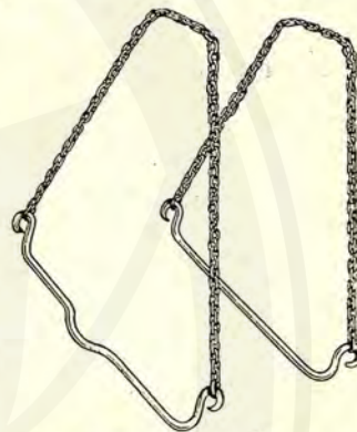
FIG. 35.—SLINGS FOR LIFTING ENGINE FROM CHASSIS.
