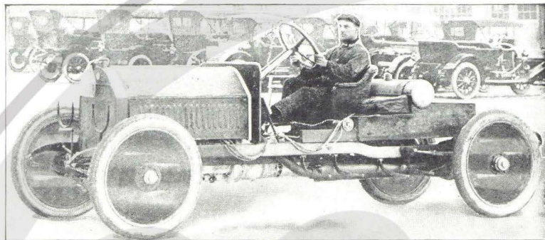
Each Chalmers chassis is tested in the "stripped" form. To compensate for the difference in weight, heavy cast iron ingots are carried in the rear of the chassis. The picture shows a Chalmers "Six" in the road test.
