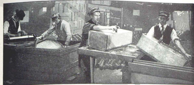
Each Chalmers radiator and gasoline tank is first filled with air under pressure and then submerged in water. One bubble rising to the surface means the rejection of the part under test.
