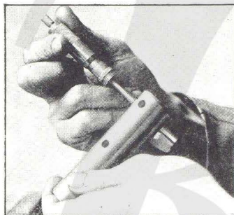
A micrometer is capable of measuring as fine as 1-10,000 part of an inch. The micrometer test is used on every moving part of a Chalmers car. The picture shows the micrometer test of a wrist-pin from a Chalmers piston.
