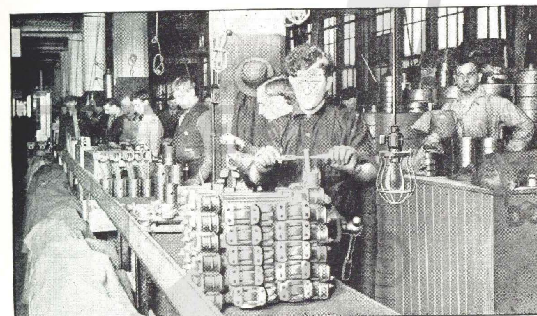
Each man in the Chalmers motor department is a specialist. The men shown in the picture are assembling connecting rods, pistons and fly wheels. They do nothing else, and as a result, their work is as accurate as human skill can make it.
