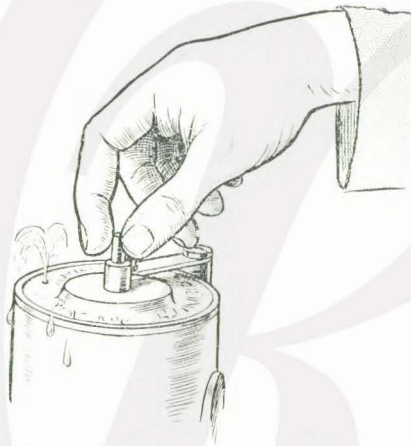
FIG. 27.—FLOODING THE CARBURETTOR.
