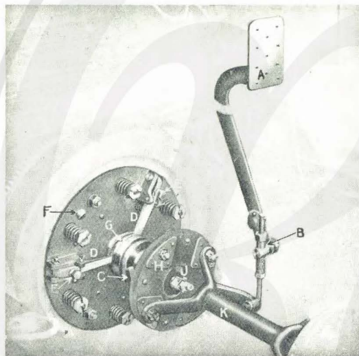
FIG. 82.—THE CLUTCH OF THE 14 H.P. "STANDARD" MOUNTED ON THE FLYWHEEL.
