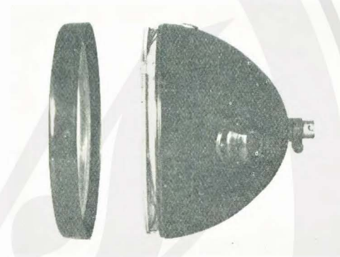
FIG. 104.—THE LATEST PATTERN C.A.V. HEADLAMP WITH A "BAYONET" FIXING FOR THE FRONT GLASS.
