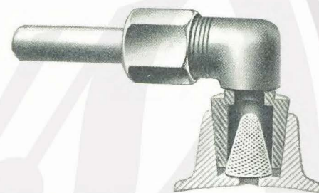
FIG. 87.—THE "THIMBLE" FILTER WITHIN THE PETROL FEED PIPE UNION OF THE AUTOVAC PETROL TANK ON THE 14 H.P. "STANDARD."
