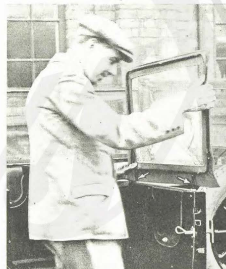
FIG. 4.—SHOWING HOW THE RIGID-FRAMED SIDESCREENS OF THE "COLESHILL" TWO-SEATER AND "KINETON" FOUR-SEATER FIT IN POSITION.
