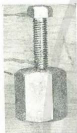
FIG. 80.— A SPECIAL TOOL PROVIDED FOR DRAWING OFF THE REAR HUBS.
