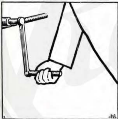
THE RIGHT WAY. It should be remembered also that the engine must always be started by PULLING THE STARTING HANDLE UP and not by pressing it down.
